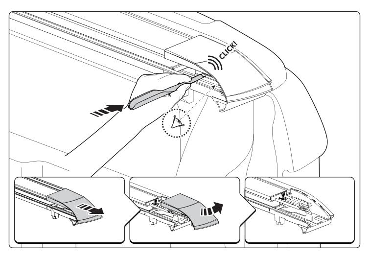
Use the multi tool to remove the plastic covers on the side profiles.
