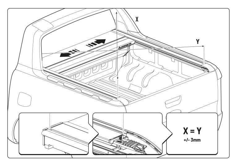
• Ensure the cross measurements are identical.
